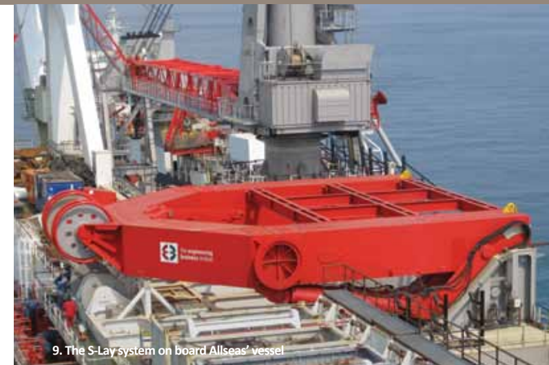
8. IHC EB supplied the pipe-handling and working stations for Allseas' S-Lay system
